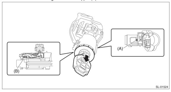
(3) Insert a flat tip screwdriver from the steering lock frame hole (A), and release the claws to pull out the key cylinder.
