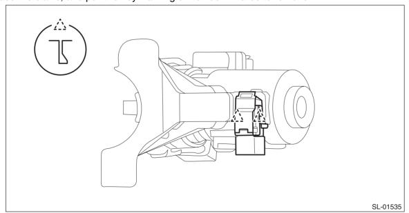
3) Remove the screws and remove the key lock solenoid.
