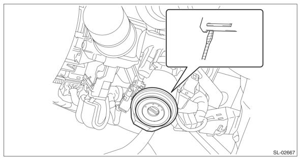
2) Release the claws, and pull the key warning switch downwards to remove.
