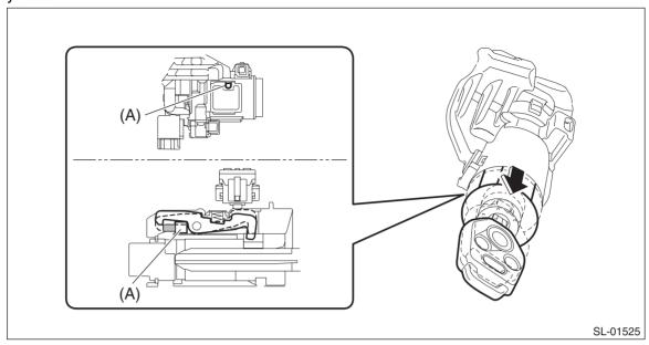
5) Release the claws and remove the ignition switch assembly.
